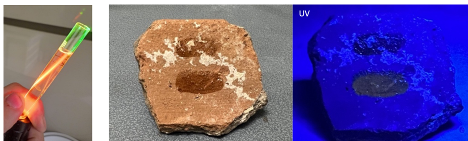
Figure 1. Carbon dots in solution under green laser excitation;
